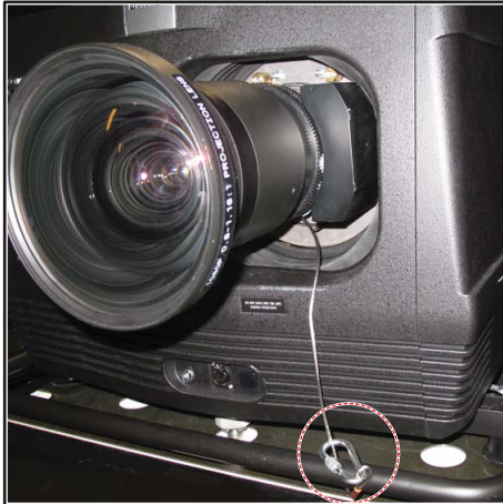
Image 1-7 Example using the bottom carrying handle
