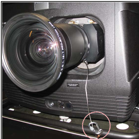
Image 1-9 Example using the bottom carrying handle
