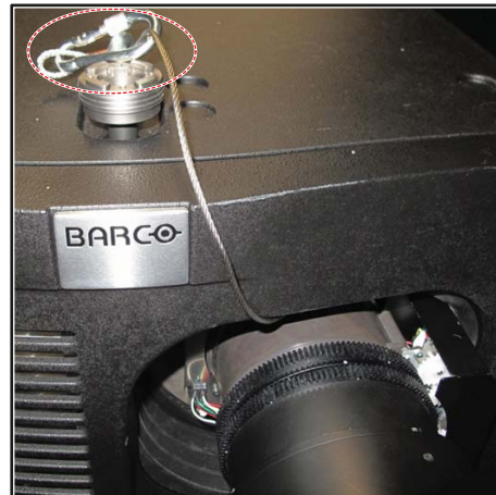
Image 1-10 Example using the hoisting eye
